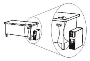
Insert the receiver's captive USB cable connector into an available USB receptacle on your computer.
